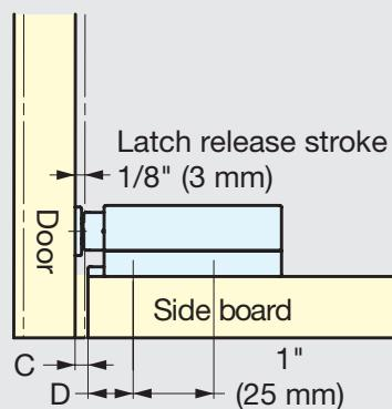
Please make sure there is a "C Clearance" on the side board. It makes the installation easier to align the edge of the body to the edge of the side board.
